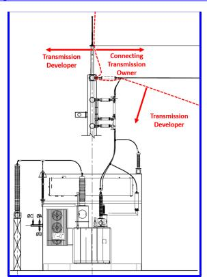
Figure C-3: Representative Substation A-frame Interconnection Drawing
